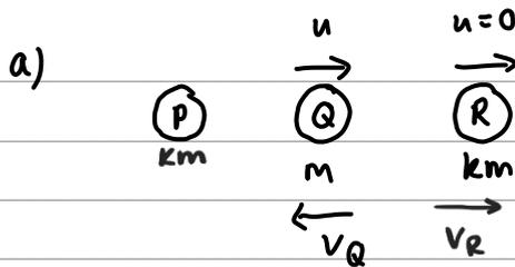
second collision occurs if direction of  $Q$  is reversed ( $v_Q > 0$ )
